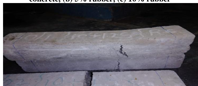
Fig.6. Failure of the concrete prisms (a) 10% Rubber with 1.2% of steel fiber
