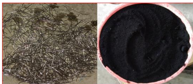
Fig.1. Hooked end steel filaments and 30 mesh crumb rubber
