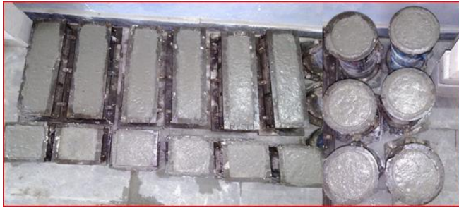
Fig.3. Casting of specimens
