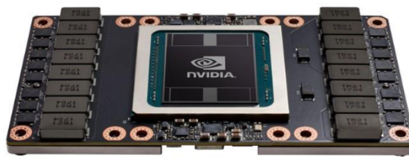
Figure 1. NVIDIA Tesla V100 SXM2 Module with Volta GV100 GPU [16]
