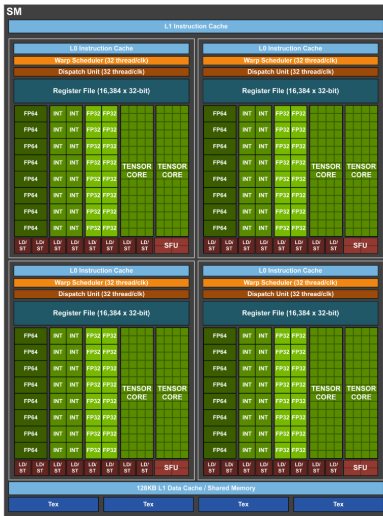
Figure 3. NVIDIA Volta GV100 SM [16]
