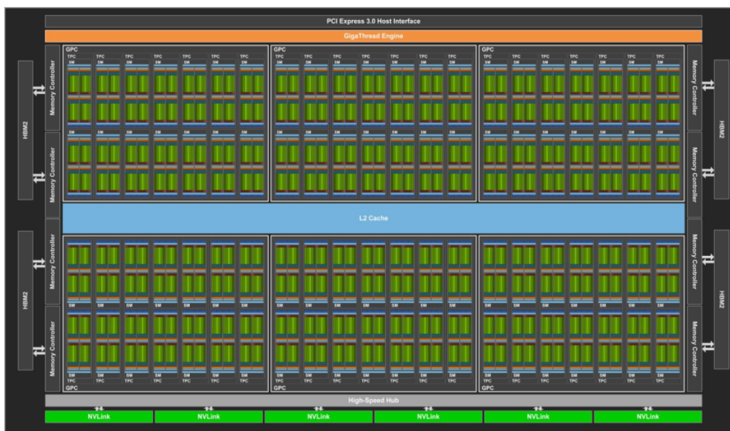
Figure 2. NVIDIA Volta GV100 GPU with 84 SMs [16]
