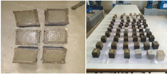
Fig.3Mortar cube SAI Test specimen
