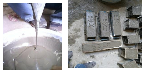
Fig.2 Marsh cone flow and SCC specimen
