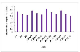
Fig.9.Flexural Strength at 7 days.
