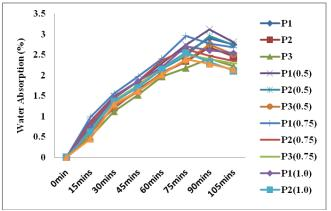
**Fig.5.Water absorption percentage of different mixes. Compressive Strength Test:** Test results of 7 days and 28 days are tabulated in table.IX.
