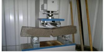
**Fig.8.Flexural Strength test**
