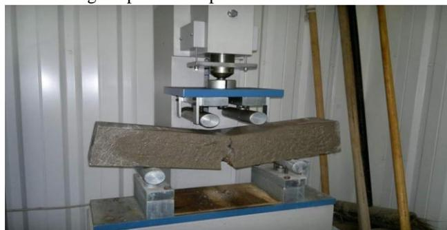
Fig.8.Flexural Strength test
