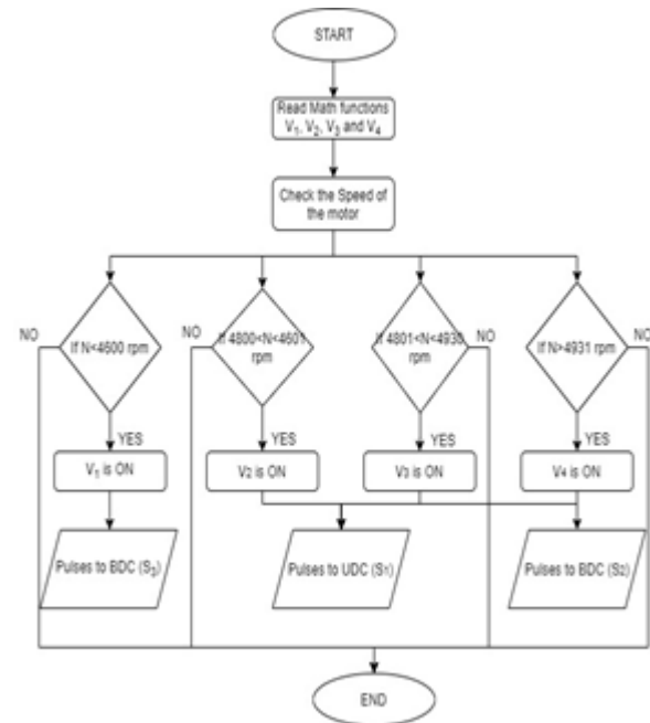
Fig. 7. Flow chart for MFB Controller implementation.
