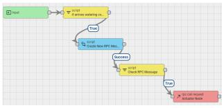
Fig. 4. A rule chain for automatic irrigation.
