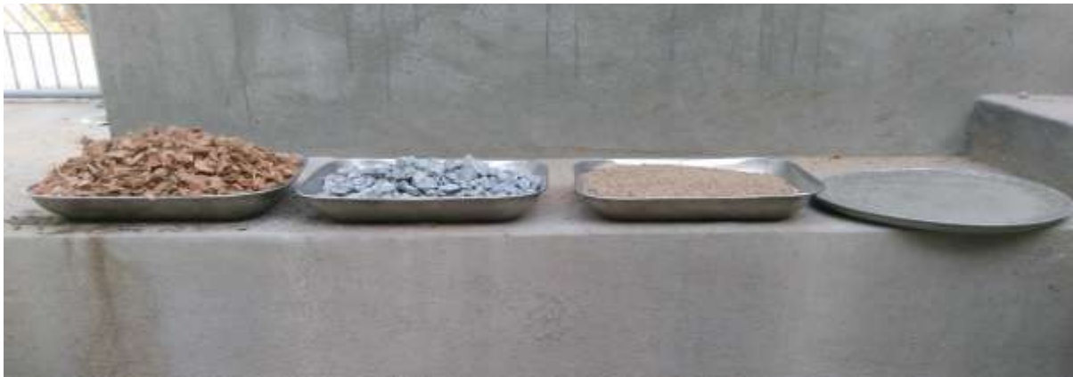
Figure 4.1 Coconut Coir Fiber Aggregates, Natural Coarse Aggregates, Fine Aggregates and Cement
