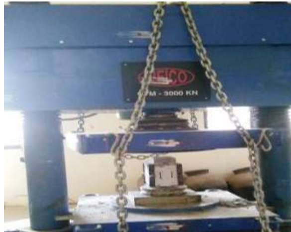
Figure 4.2 Testing of Specimen for mode-II shear
