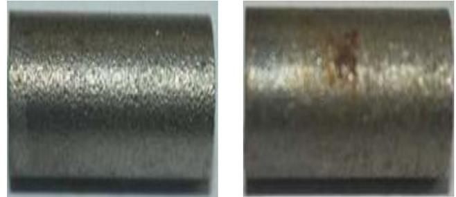
**Figure 1(a). Laser sintered Inconel 718 component before corrosion**
