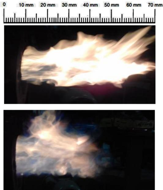
**Fig.6. Flame length with and without pulsation**
