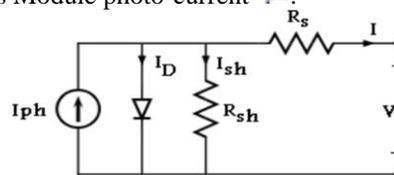
Figure 1 PV-Cell Equivalent Circuit
