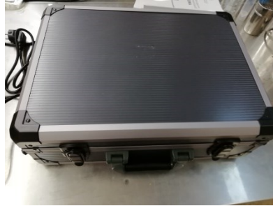
Figure 5-8: Battery back that can be used for providing power autonomy to the MIMS prototype of about 2-3 hours in the field.
