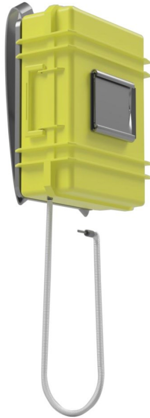
Figure 4-6: Design of the RESCUE-MIMS that can be used as a handheld or back-pack device with penetration capabilities.
