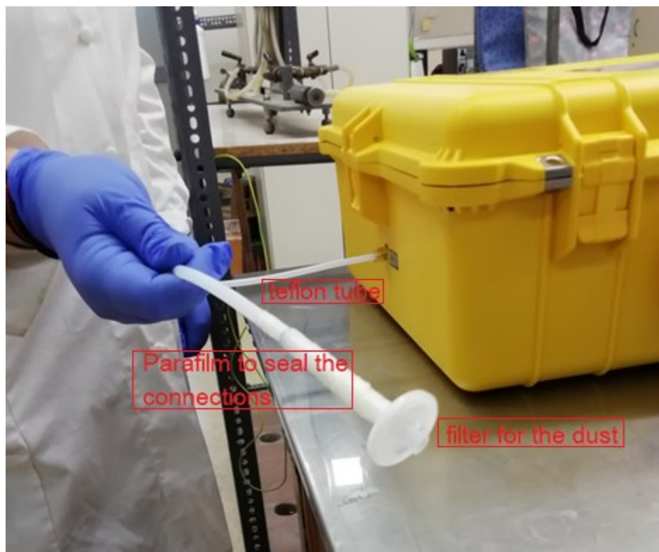
Figure 4-7: Preliminary set-up of the penetration sampling probe; in front of the teflon tube a filter has been adjusted in order to protect the instrument from the dust; a parafilm tape was used to seal the connections.
