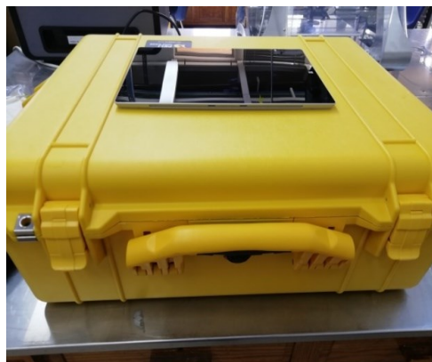
Figure 5-4: The RESCUE-MIMS peli-box with a PC laptop to display the data recorded on-line.
