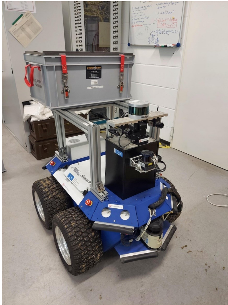
Figure 5-7: Preliminary testing on how to mount payloads on the SeekurJr robotic platform by DFKI (Provided by DFKI).
