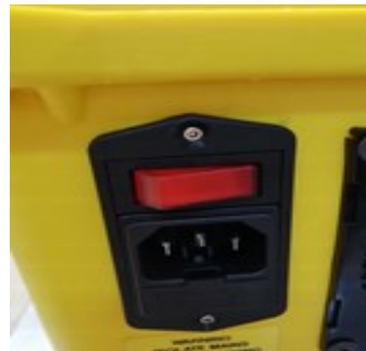
Figure 3-4: The power switch of the MIMS is at the right side of the peli-case.
