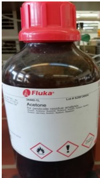
Figure 2-5: Standard solution of acetone with purity >99.5% for testing the RESCUE-MIMS
