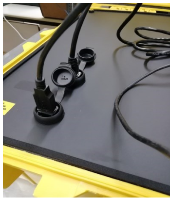
Figure 3-1: The two cables for connecting the PC with the MIMS device are plugged in the inner part of the peli-box.
