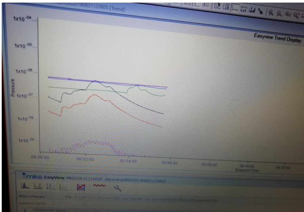
Figure 3-17: Intensities' profiles of target compounds masses: 43 and 58 for Acetone (black and orange, respectively), mass 78 for Benzene (pink), mass 18 from Water Vapours (blue), mass 40 for Argon (purple) and mass 44 for Carbon Dioxide (Green), displayed on-line by the MIMS.
