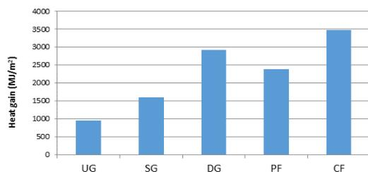
**Figure 16 Useful Heat gain for different geometry of solar air heater**
