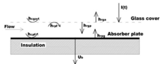
Fig. 4 Cross sectional view and nomenclature
