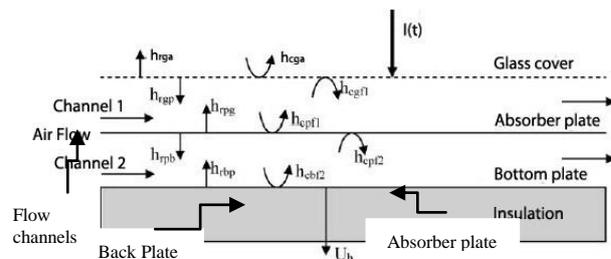
Fig 6 Cross sectional view and nomenclature
