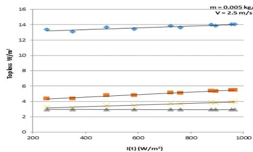
**Figure 12 Top loss for different type of SAH**
