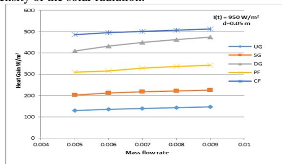
**Figure 13 Effect of mass flow rate on useful heat gain**
