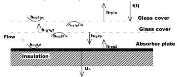
**Fig.5 Cross sectional view and nomenclature**
