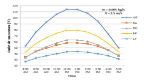
Fig. 10 Hourly variation of outlet temperature
