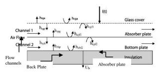
Fig 6 Cross sectional view and nomenclature
