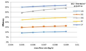
Fig 14 Efficiency variation with mass flow rate
