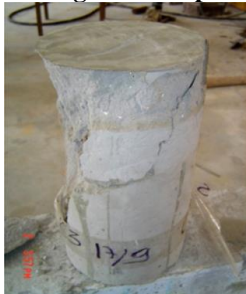
Fig. 9. The failure sample during a compression test
