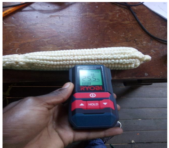
Fig. 3. Sample maize cobs (left) and moisture meter (right) measuring the moisture content of one of the dehusked maize cobs
