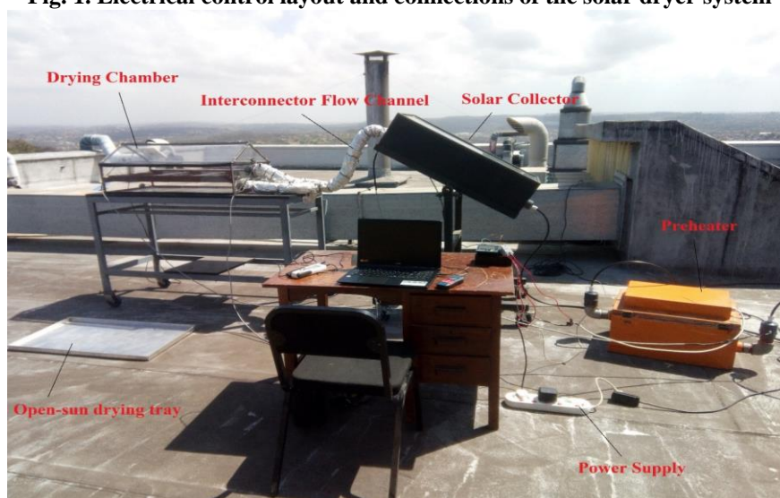
Fig. 2. Complete experimental setup of the solar dryer system
