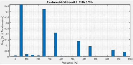
Fig. 17 THD source voltage with 3- level inverter system
