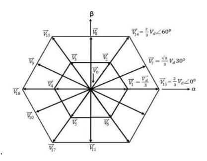
Fig.3. rotating equivalent space vector in three phase sinusoidal systems
