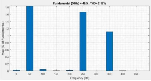
Fig. 28 THD source current in conventional system using machine load
