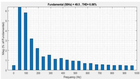
Fig. 14 THD grid voltage with conventional system
