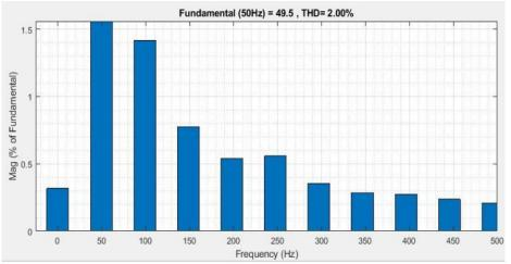
Fig. 31 THD source voltage with three level inverter systems using machine load
