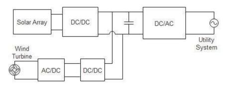
Fig.1. Distinct circuit topologies for the wind and SPV hybrid system with utility grid
