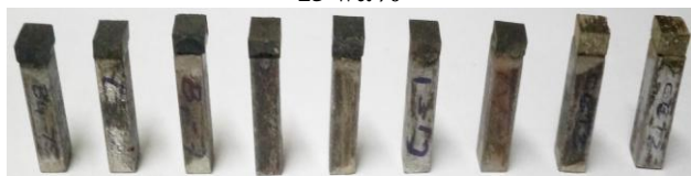
Figure 6. ASTM G 99-95 standard wear test Specimens
