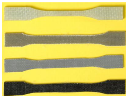
ASTM 790 Tensile test Specimens
