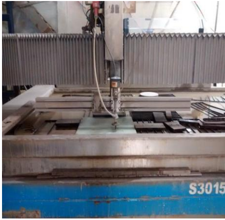
Figure. 3. Abrasive water jet machine
