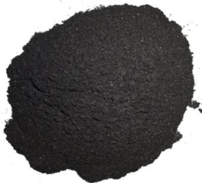
Graphite Powder (Particle Size 66 Microns)
