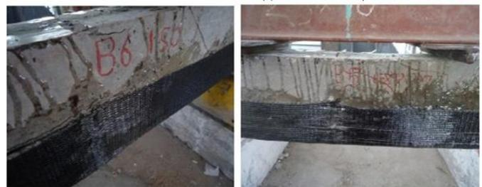
**Figure 3.4 Carbon fiber Retrofitted beam with resins (ISO, Epoxy, GP)**
