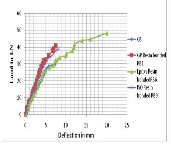
Figure 4.4 Load Vs Deflection for Controlled and Retrofitted beams with CFRP Laminates (ISO, Epoxy, GP)
