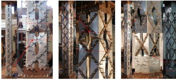
(a) Model-A (b) Model-C (c) Model-B (d) Model-D Fig 4: Failure buckling mode in the test models [7]
