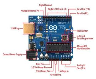
Fig.3 Arduino board
