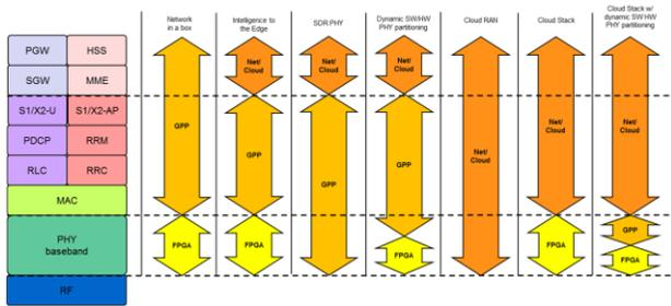
**Figure 9.** Virtual mobile network function splitting and deployment
