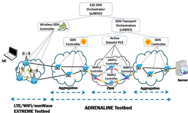
Figure 3 Integration of ADRENALINE and EXTREME testbeds.
