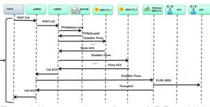
**Figure 4** Message exchange diagram of E2E provisioning services between ADRENALINE and EXTREME Testbeds.
