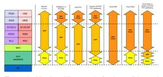
Figure 9. Virtual mobile network function splitting and deployment
