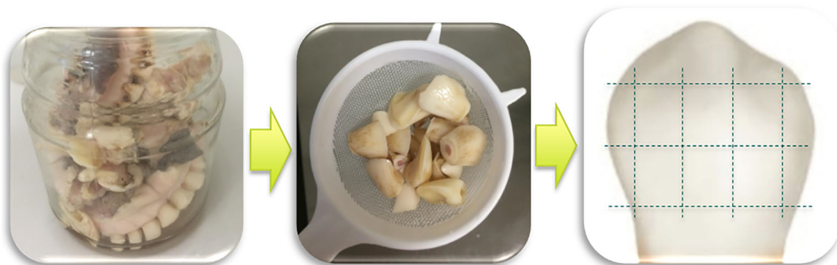
FIGURE 3 Preparation of bovine enamel blocks
