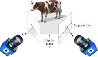
Fig. 3. Epipolar geometry
