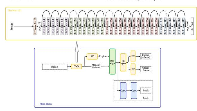
Fig. 5. Detailed architecture of the Mask R-CNN network
