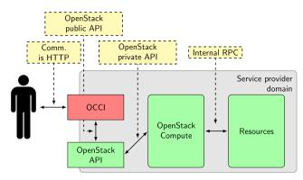
Fig. 3. OCCI place in a provider's infrastructure, following ooi's architecture. Instead of using the private APIs, OCCI requests are translated to native OpenStack requests. Boxes in yellow explain the type of communication being made, green depicts the OpenStack components, red the OCCI interface. (For interpretation of the references to color in this figure legend, the reader is referred to the web version of this article.)
