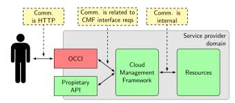
Fig. 2. Proposed OCCI's place in a provider's architecture according to the standard. Boxes in yellow explain the type of communication being made, green depicts the Cloud Management Framework components, red the OCCI interface. (For interpretation of the references to color in this figure legend, the reader is referred to the web version of this article.)
