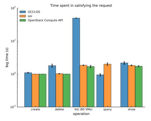
Fig. 4. Performance comparison between both OpenStack implementations, using a logarithmic scale in the *Y*-axis. The listing of the running instances has been made against an infrastructure running 80 instances. Standard error is represented in the error bars. Note that the *query* operation for OpenStack is not applicable, as it is OCCI specific and there is no equivalent in OpenStack.
