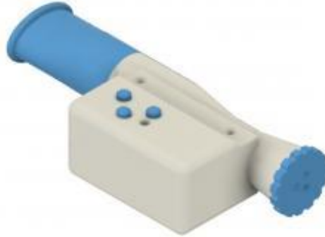
Spirotroller gaming [J] Controller measuring the flow and pressure, 3d-printed, Bluetooth, three buttons Direct use Actively developed
