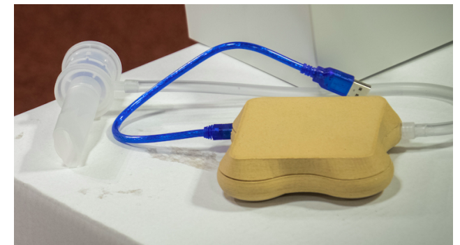
3D organic box [B] Controller measuring the expiratory pressure, 3d-printed, USB, 1 LED Use with mouthpiece Prototyped
