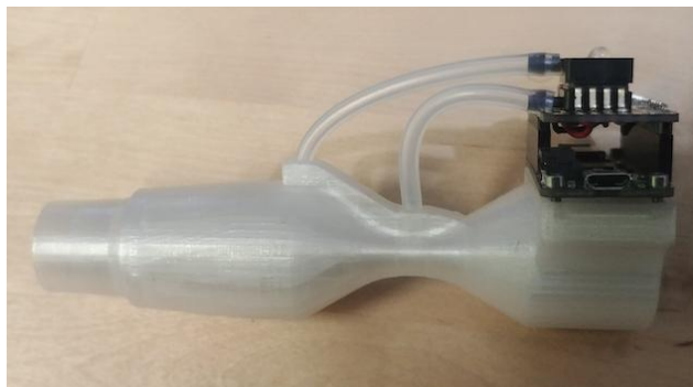
Spirotroller [G] Game controller measuring the expiratory flow, 3d-printed, Bluetooth and USB, one button Direct use Prototyped
