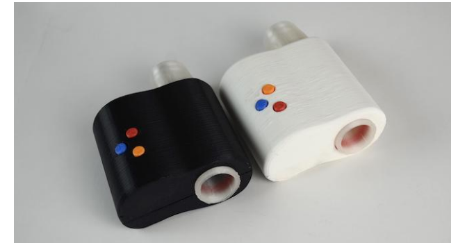
Spirotroller enhanced [H] Game controller measuring the expiratory flow, 3d-printed, Bluetooth and USB, three buttons Direct use Prototyped and tested
