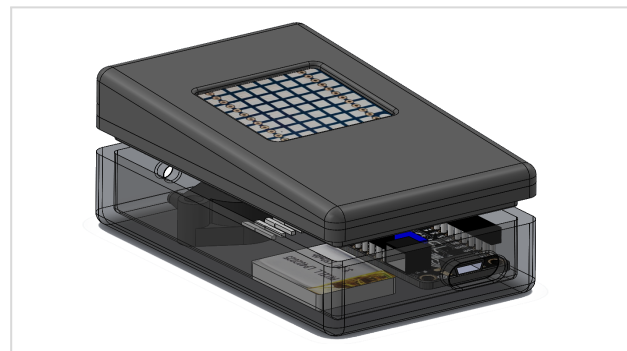
Led box [C] Controller measuring the expiratory pressure, 3d-printed, Bluetooth and USB, 8x8 LED matrix Use with mouthpiece Prototyped
