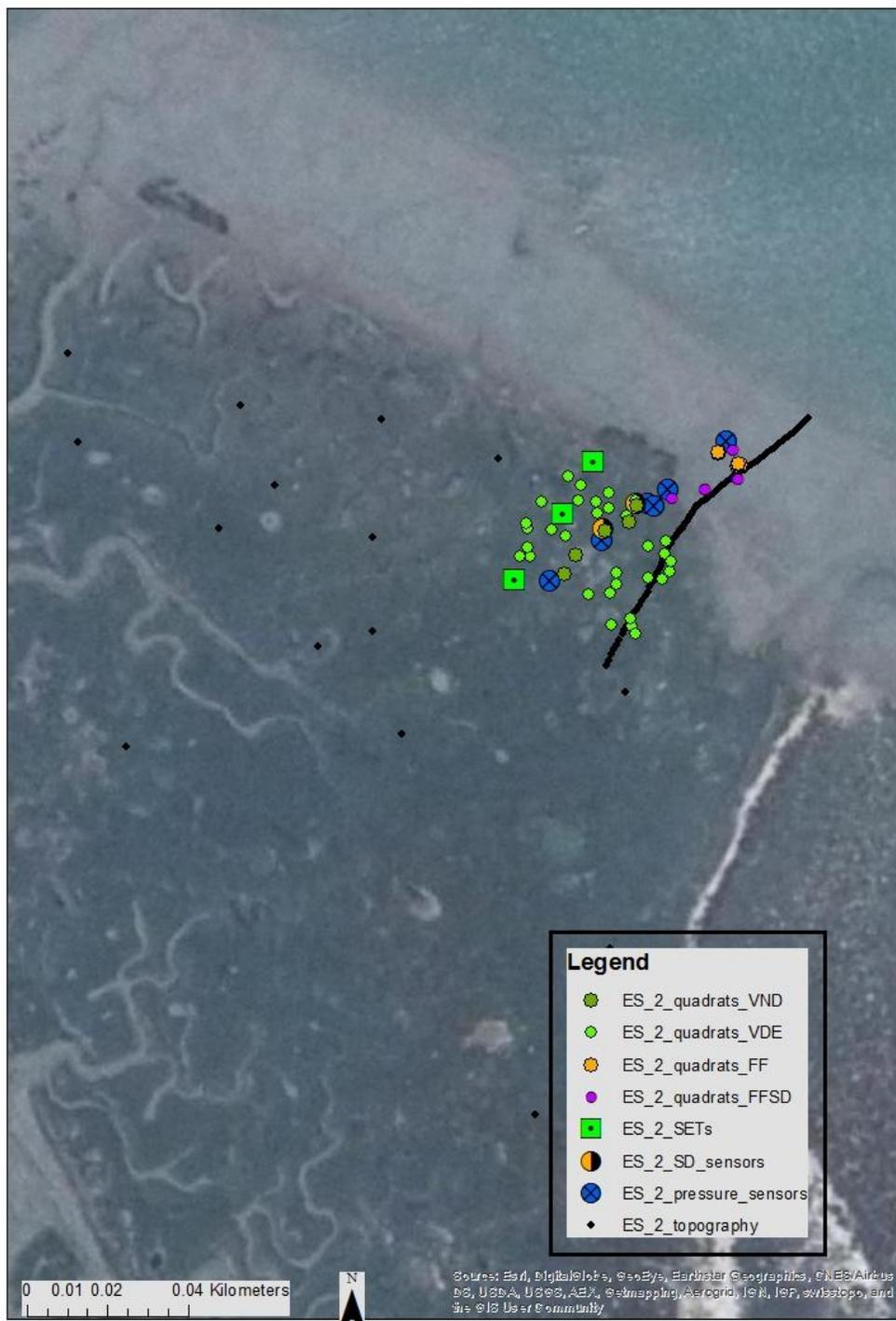
Figure 4: Locations of topographic surveys, monitoring equipment and sampling quadrats deployed at ES Y2 site
