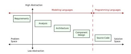
Figure 4.1: Phases of the software development lifecycle, abstraction levels and language types. *Source*: Author's drawing based on Berg *et al.*'s [BBM05] image.
