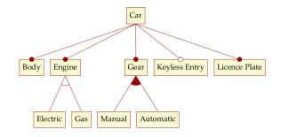
Figure 6.3: Sample feature model. *Source:* Author's drawing, modified from a Czarnecki and Wasowski diagram [CW07].
