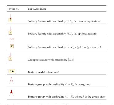
Figure 6.2: Symbols used in cardinality-based feature modeling. *Source:* Author's drawing, based on Czarnecki and Helsen [CHo6]
