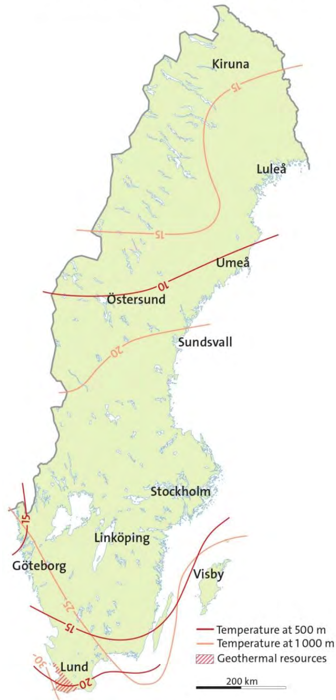
Figure 9. Temperature of the uppermost crust in Sweden, at 500 m and 1000 m depth (Hurter and Haenel 2002)
