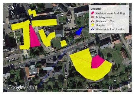
Figure 2: Land and building constraints for the geothermal project of Crèvecoeur-le-Grand Hospital.
