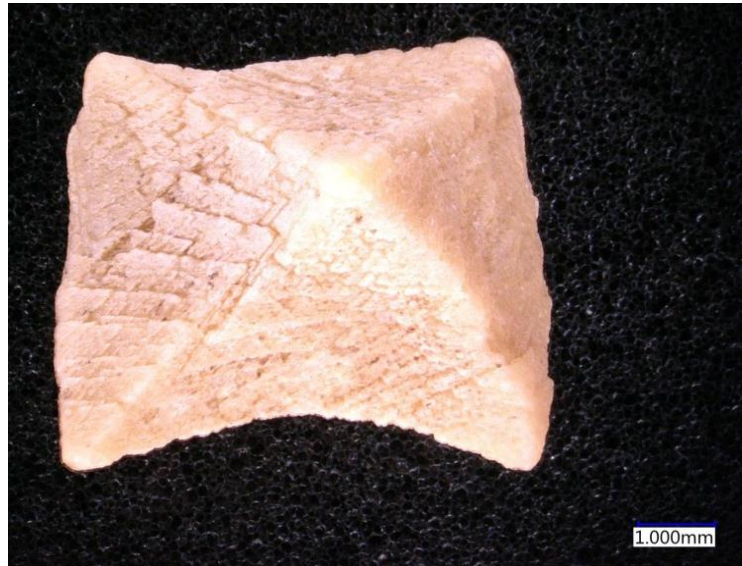
Figure 4-5: Pyramidal shape with stepped surfaces. This morphology is exclusively associated with blocky texture in transmitted light.
