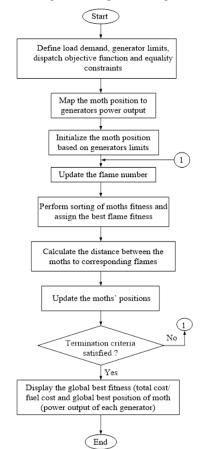
Figure 1: Moth flame optimization algorithm flow chart
