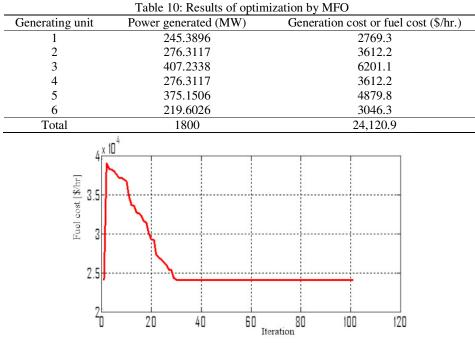
Figure: 4 Convergence curve of ELD at load demand of 1800 MW
