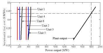
Figure 2: Incremental fuel cost versus the power outputs of the generators and the plant
