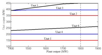
Figure 3: Output of each generating unit versus the total plant output
