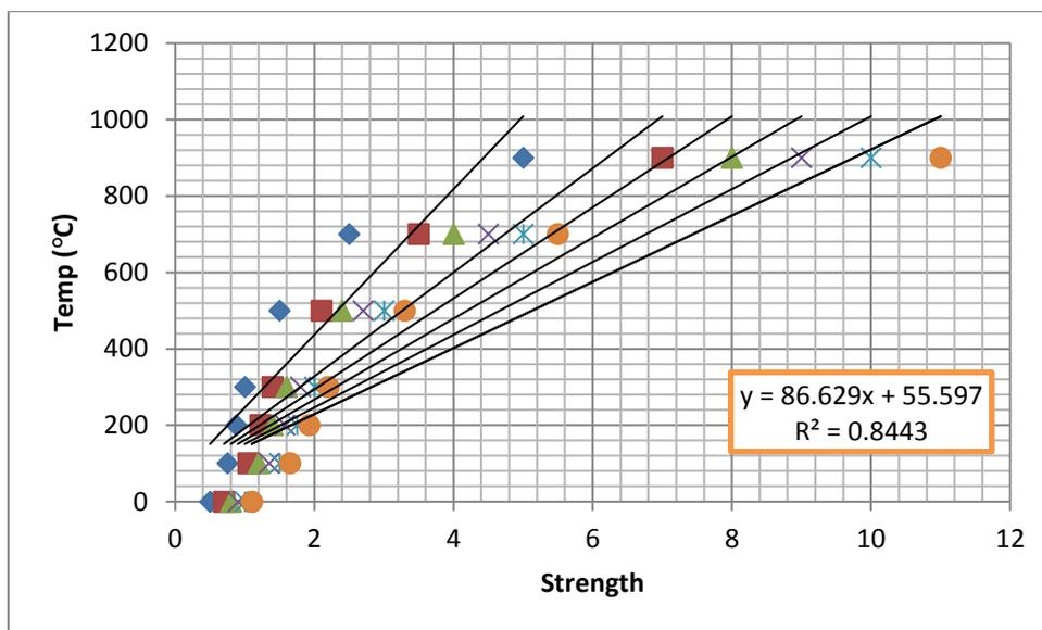
Figure 11. Relationship between unconfined compressive strength and heat
