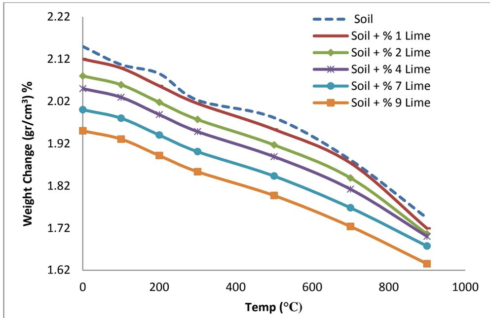
Figure 6. Weight changes of soil samples subjected to heat for samples containing lime
