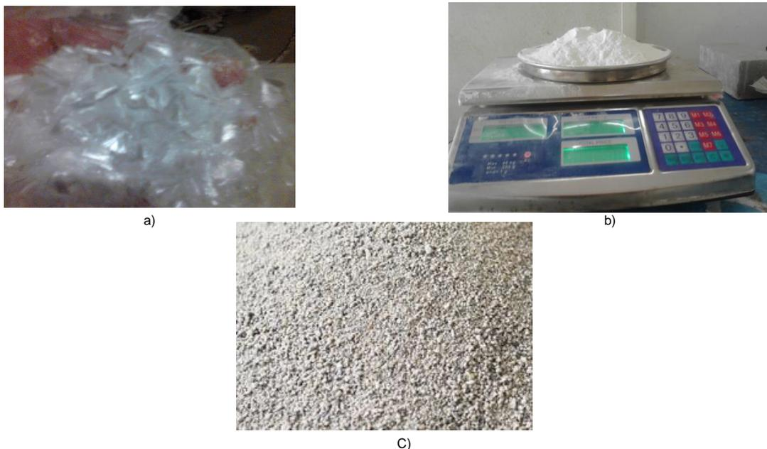
**Figure 2.** Materials used in this study (a) fibers, b) lime, c) bentonite
