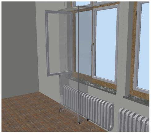
**Figure 2:** CAD model of a movable (rollable) draught projection system built of polycarbonate double-webbed sheets, aluminium corner profiles, and furniture casters for historic-building-preservation, draught-reduction and the thermally comfortable introduction of fresh air from a window to the floor (via fully or partially opened turn-only window or laterally tilted window). The window remains fully functional and can be closed outside lesson time so that no additional heat loss occurs.
