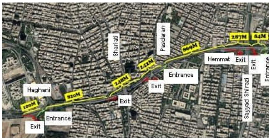
Figure 11. Distances between access points based on the Enactment No.32 of the supreme council for traffic coordination of Iran ministry of road and urban development
