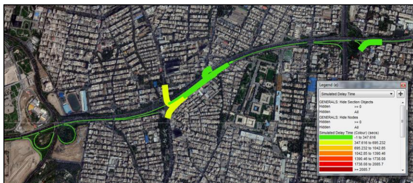
Figure 7. Graphic delay index (an increase of lanes number and ramp metering solution) –After calibration
