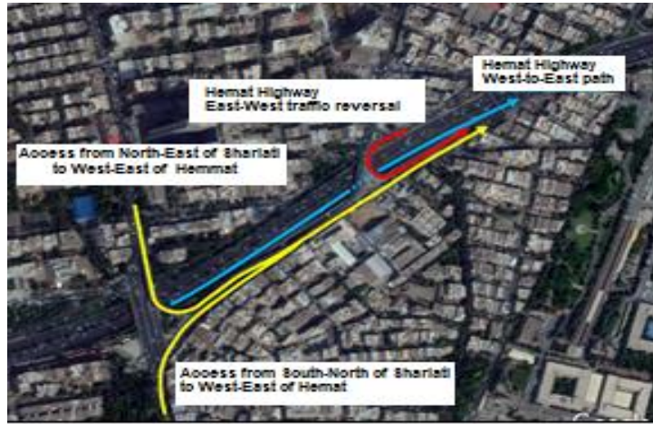
Figure 3. Interference of high traffic between West-East of Hemmat path and High traffic of entrance ramp after Pasdaran passage
