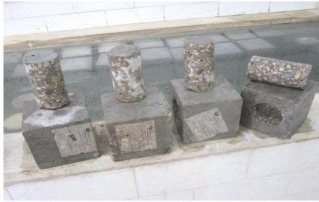
Figure 9. Core taken from cube specimens to measure water absorption
