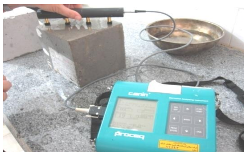
Figure 11. The method to measure electrical resistivity of the sample
