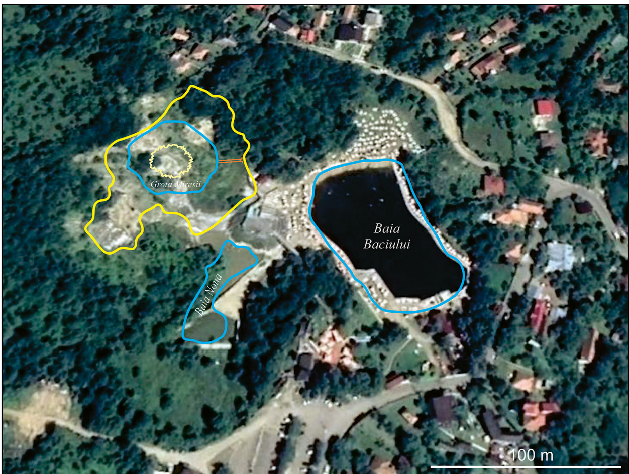
Fig. 8. Google Earth image of the Salt Mountain area ( August 5, 2020 , 47 years after the general view of 1983 – photo 7c – was taken). The outlines of the 1987 Salt Mountain outcrop (in yellow), the inner lake formed by the collapse of the bell-shaped salt mine (in blue) and of the upper aperture of the Bride's Cave (in yellow) are superimposed on the background provided by the GE image. A gallery to the inner lake (visible in Fig. 7a), dug in the salt wall, is shown with brown lines. The contour lines are taken over and modified from Bulgăreanu et al. (1987) and Bulgăreanu and Cehlarov (1993). For orientation and comparison, on both images (Photo 7c and GE image) it is easy to identify the street that borders the reserve to the north-east and north.
