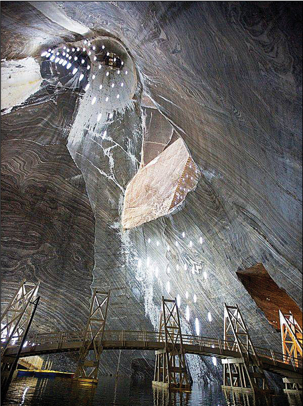
Fig. 15. The modernized Turda salt mine, showing the older, bell-shaped Terezia mine, with its access wells on top and a newer trapezoidal gallery cut in one of its walls. Tight, isoclinal or sheath folds are seen in the walls, as well as stalactites and salt crusts, formed in areas of water circulation on fractures and access wells. Photo courtesy Călin-Andrei Stan.
