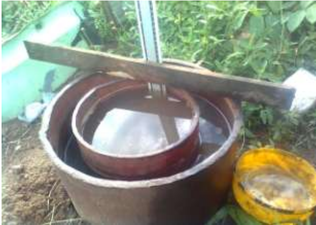
Figure 1: Infiltration study with a concentric double ring infiltrometer.
