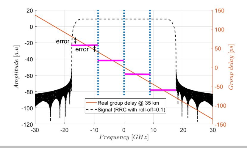
Can the group delay be compensated in a "quantized" way?
