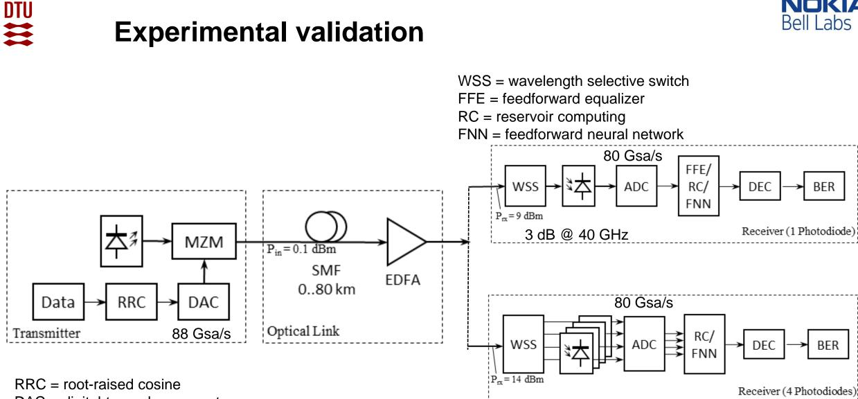
DAC = digital-to-analog converter MZM = Mach-Zehnder modulator NOKIA
