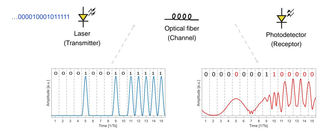
Fiber dispersion + direct-detection = inter-symbol interference
