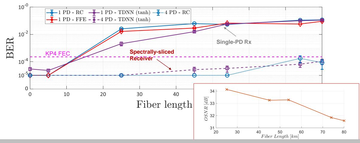
Spectral-slicing + equalization significantly enhances the transmission reach.
