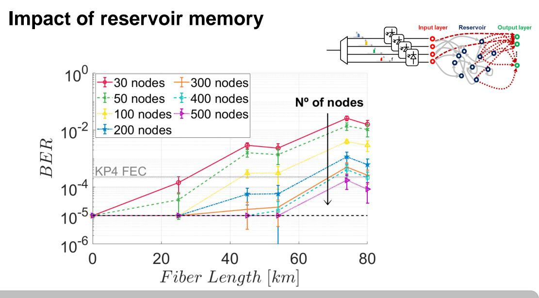
The equalizer memory needs to be adjusted for the specific transmission distance.
