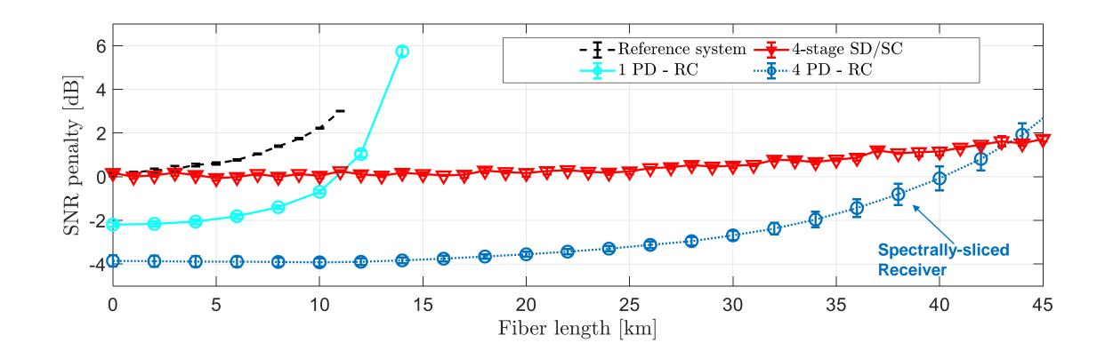
Significant increase in transmission distance, comparable with 4-stages SD/SC.
