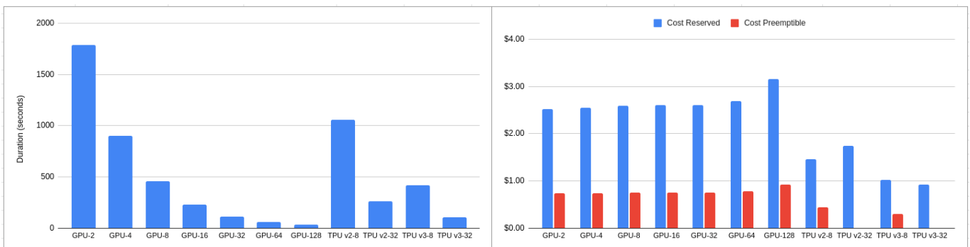
Results from one of the sample workloads taken for evaluation on Google Cloud Platform. Specifically, it shows the distributed training of a 3DGAN for fast simulation. The left-hand graph shows the raw results with up to 128 parallel GPUs (achieving linear scaling), as well as with TPUs (up to 32 cores). The right-hand graph shows the overall cost of each run. The GPU runs show a flat overall cost, even with the larger number of GPUs providing a speedup of over 52x. The TPU runs show that this type of resource is not only efficient, but it is also the most cost effective for this particular workload.
