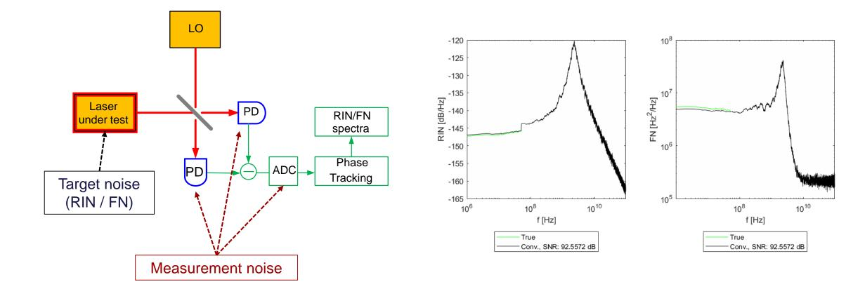
RIN: relative intensity noise, FN: frequency noise, PD: photodetector, ADC: analog-to-digital converter
