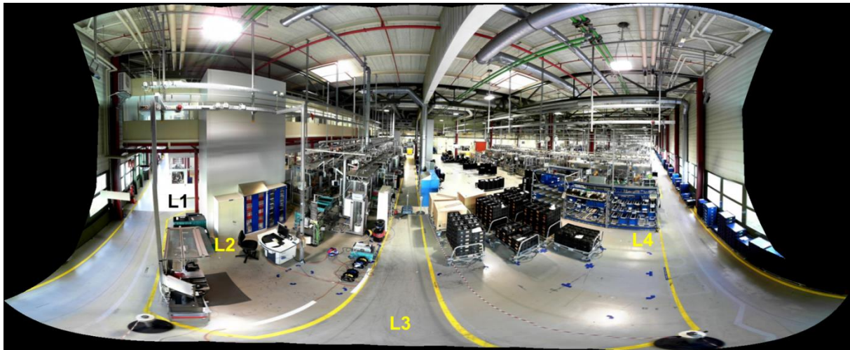
Figure 19 - Composite picture taken by the channel sounder at the TX and the different measurement lines (L1 to L4)
