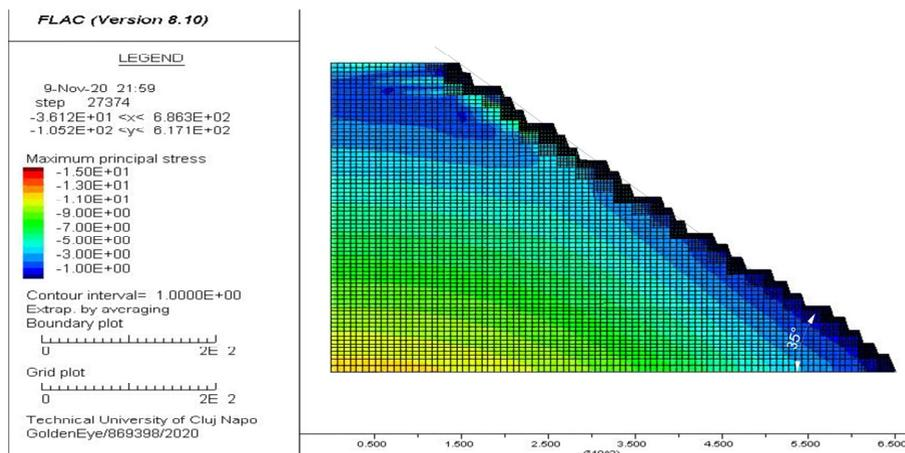
**Fig. 3.** Mesh generation with calculated  $\sigma_1=8.7$  MPa (24 berms)
