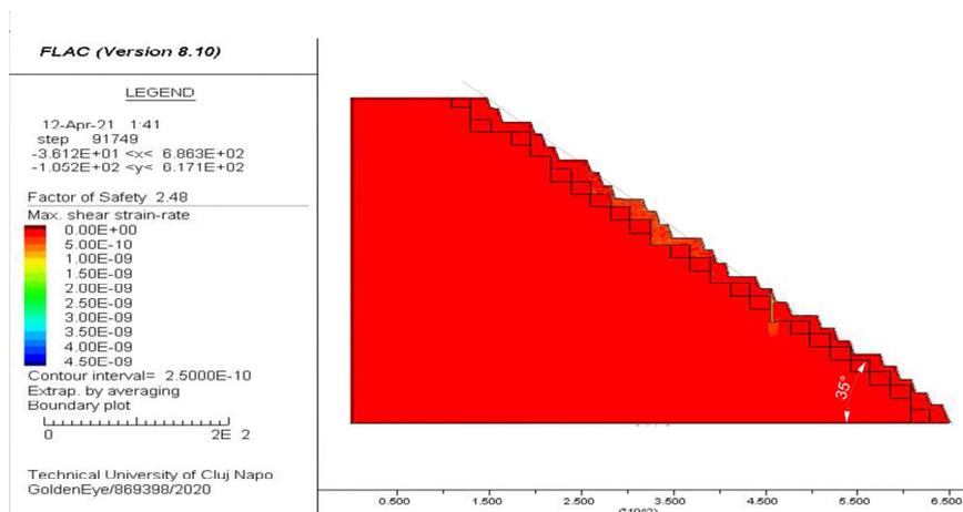
**Fig. 4.** FoS=2.48 and Max. Shear strain-rate (24 berms)
