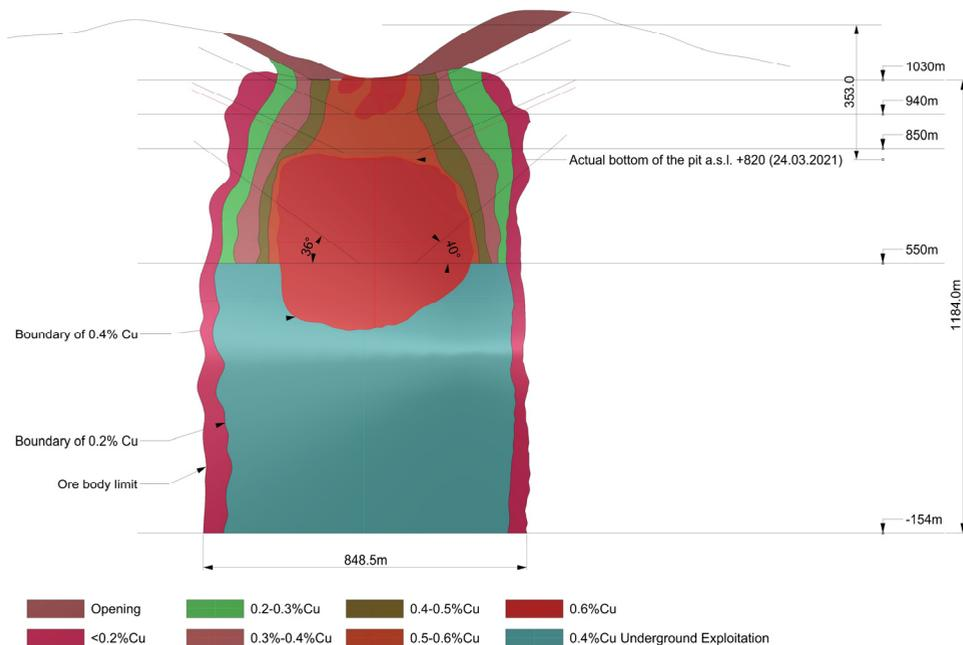
**Fig. 1.** Ore body of Rosia Poieni mining field, after [3].
