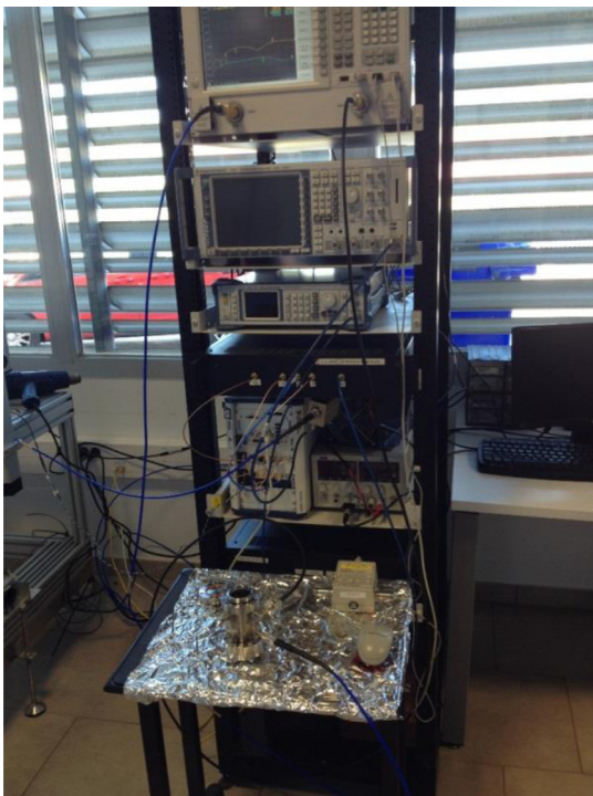
Fig. 14. One BPM under RF and electrical characterization checks in the laboratory.
