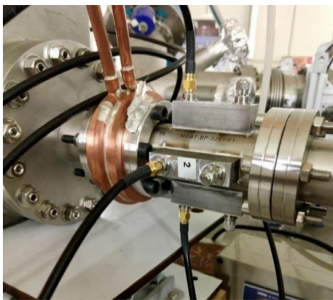
Fig. 20. BPM installed and protected with collimator for vertical test at IPHI beamline (left) and horizontal/vertical beam position changes for 30 consecutive pulses.
