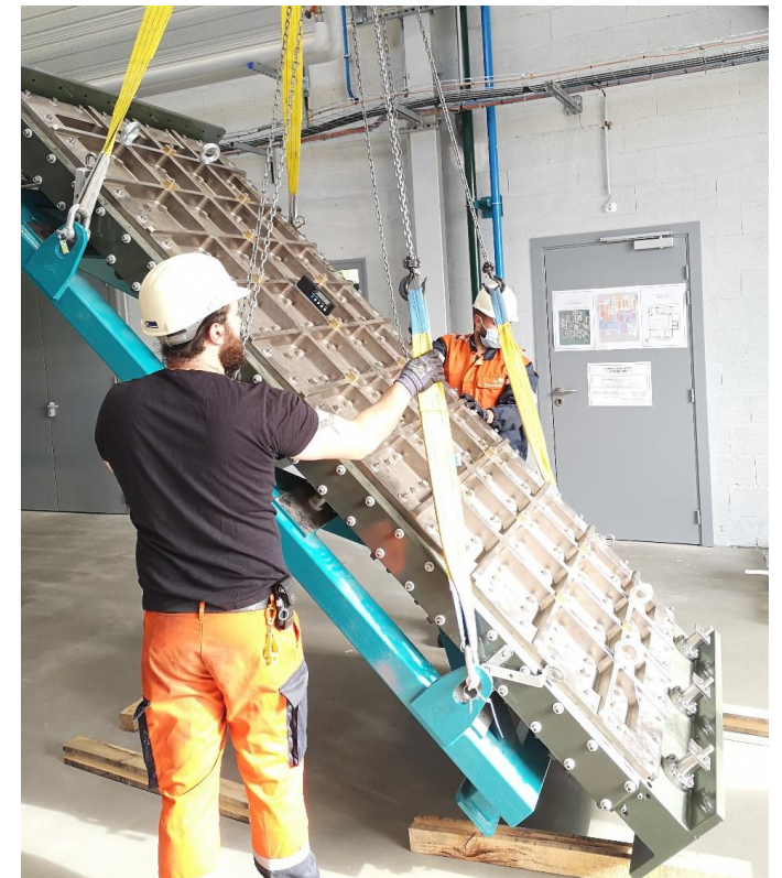
Electrowinning cell for 100 kg iron plate production.
