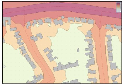
Figure 9: Example of noise level contour polygons generated using recommended methodology
