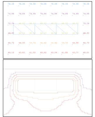
Figure 7: Grid with quiet points inside building results in 5 dB contours in front of building which is not realistic
