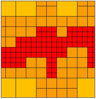
**Figure 3:** Example of grid points (in centre of each square) that represent areas of 100m<sup>2</sup>, 400m<sup>2</sup>, and 1600m<sup>2</sup> without overlap of missing parts
