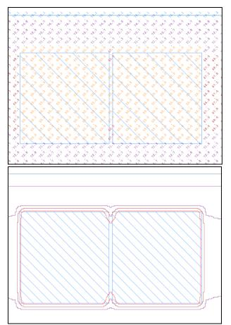
Figure 8: Grid with quiet points inside building results in 5 dB contours in front of, and behind, the buildings which is not realistic
