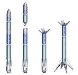
Fig. 1. Conceptual sketch of the RETALT1 spacecraft. Configurations from left to right: launch, stage separation, first stage descent, first stage landing.
