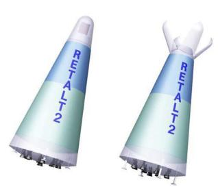
Fig. 2. Conceptual sketch of the RETALT2 spacecraft. Configurations from left to right: launch, descent and landing.
