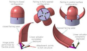
Fig. 5. Concept of aerodynamic control surface mechanism for RETALT 2
