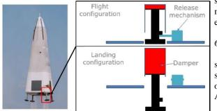
Fig. 6. RETALT 2: pneumatic cylinder
