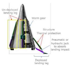
Fig. 7. RETALT 2: deployment kinematics
