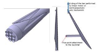
Fig. 4. RETALT1: leg structure attached to actuator
