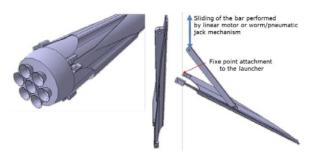
Fig. 3. RETALT1: linear actuator attachet to silidng bar
