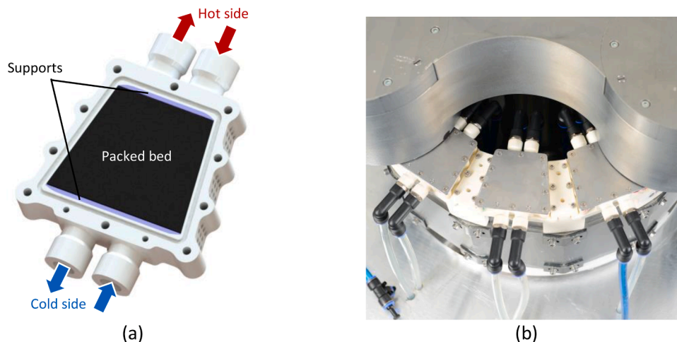
Fig. 6. (a) CAD model of the tapered bed and (b) photo of the beds installed on MagQueen.
